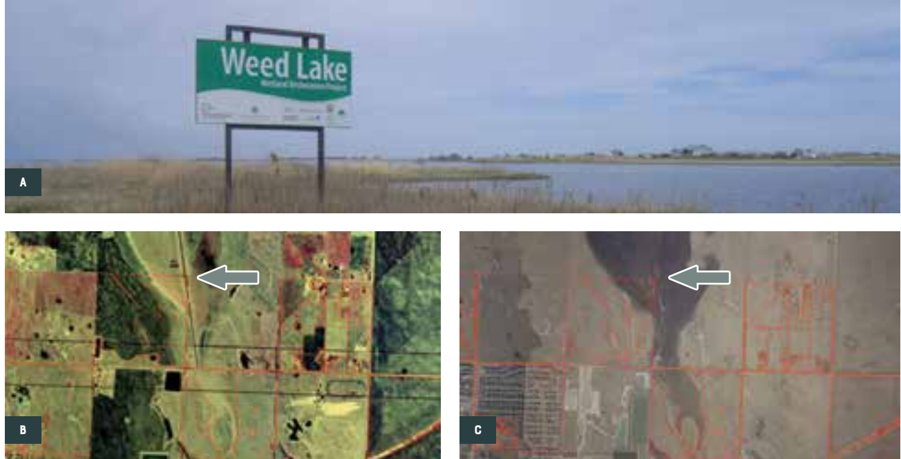
Figure 18. (A) A Ducks Unlimited Canada wetland restoration project in (B) 1985, and (C) 2011. Note the large drainage ditch (at location denoted by the arrow) in the baseline 1985 photo. The ditch is submerged, but still visible in the 2011 air photo; however, a drain plug/control has been installed and the wetland has been restored. This restoration resulted in an increase in wetland habitat area on sampled PHMP transect quarter-sections.
